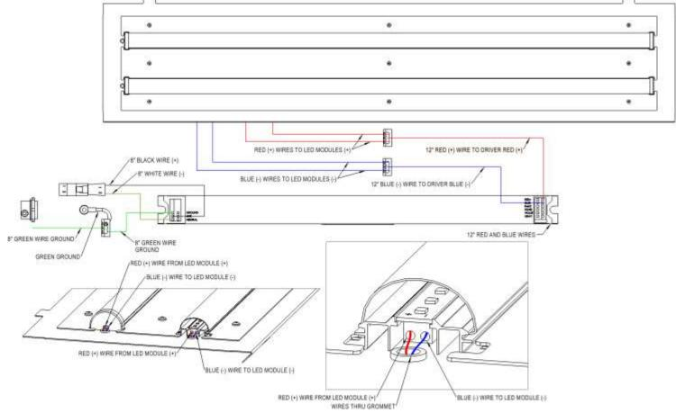
**NOTE**: THE LED DRIVER IN THIS FIXTURE IS DESIGNED TO OPERATE ON GROUNDED NEUTRAL SYSTEMS ONLY. **IMPORTANT SAFETY NOTE**: THERE IS STILL VOLTAGE INSIDE THE FIXTURE WHEN THE FIXTURE IS OPENED. **WARNING**: TO PREVENT THE RISK OF ELECTRICAL SHOCK DEACTIVATE/DISCONNECT THE POWER SUPPLY BEFORE MAINTENANCE OF FIXTURE.
