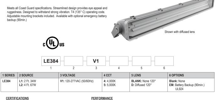
UL 844 / CSA 22.2 No.137.0 (Hazardous Location) CI D2, Grps A,B,C,D T-Codes: CI D2=T4 UL 1598 / CSA 22.2 No.250 (Wet / Damp) UL 1598A Marine Outside (Marine) Lumen Maintenance (L70) 54,000 hrs. (reported) CRI>80 -30°C to 40°C Ambient
