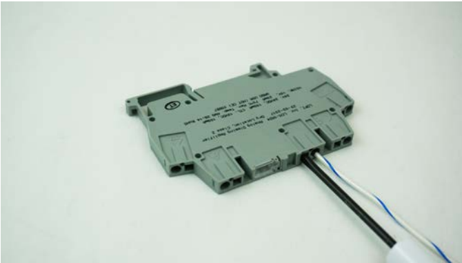
Fig 6 – Once open, keep the screwdriver inserted to keep the wire clamp open and insert the end of a wire, stripped to the length specified by the device's datasheet, into the neighboring circular access hole.
