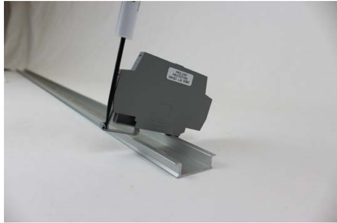
Fig. 3 – Continue pulling away and up until the latch arm has cleared the rail
