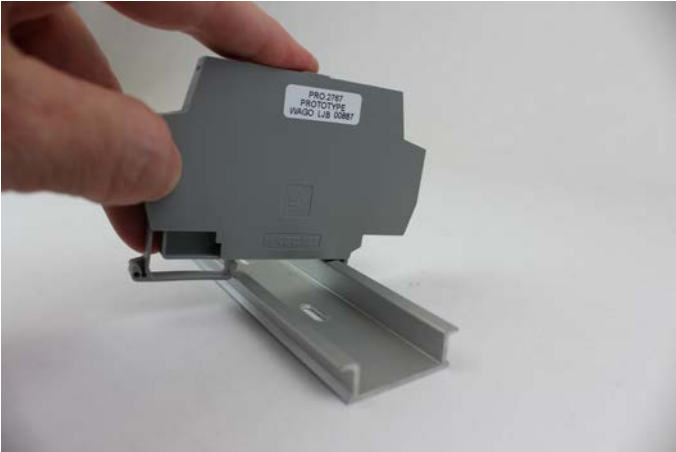
Fig. 1 – Attach the hook to the DIN rail and press straight down until device is secure.
