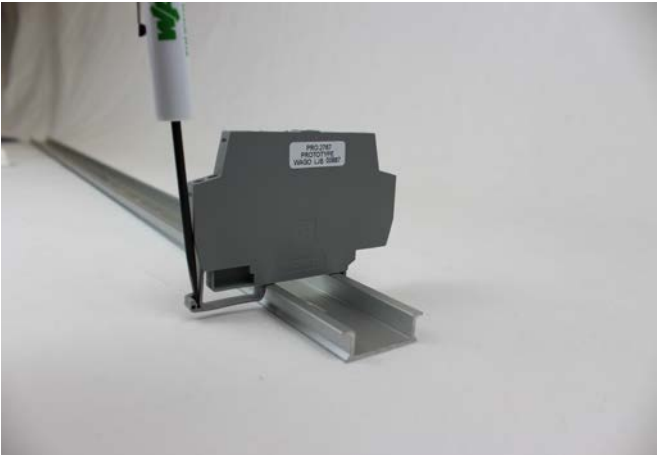
Fig. 2 – Using a small, flat-head screwdriver, apply force to the latch away from the rail
