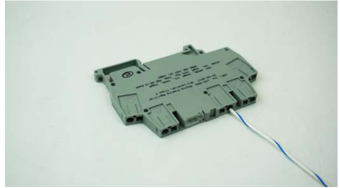
Fig 7 – Remove the screwdriver from the square access hole and lightly tug the wire to ensure proper installation.
