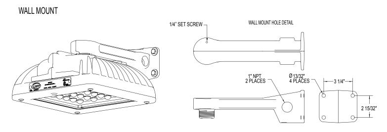
Securely tighten set screws when desired fixture orientation is achieved and the conduit connection is tight.
