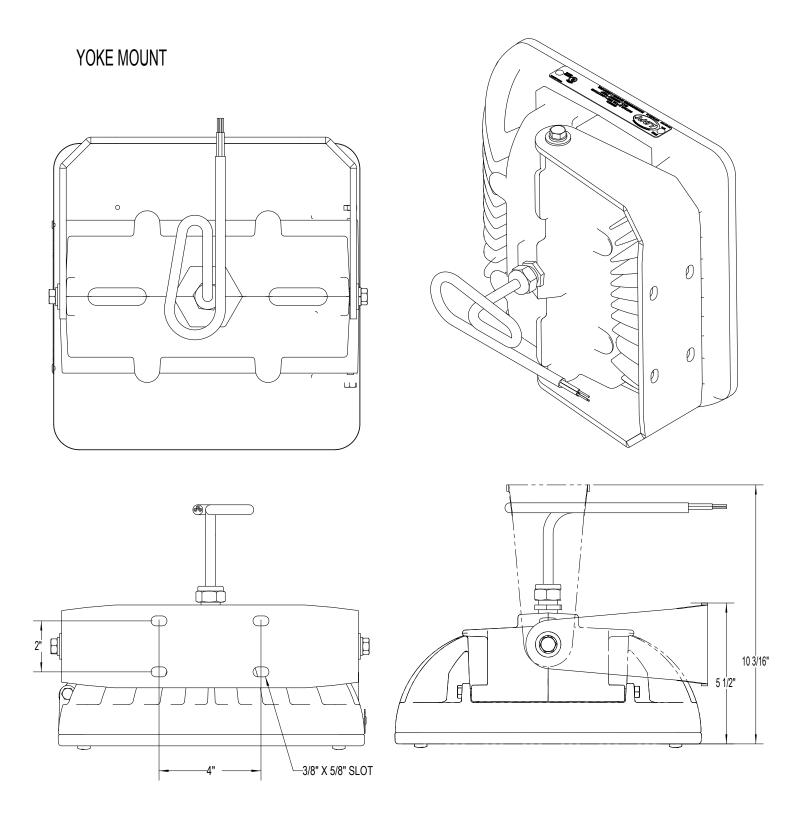
**NOTE:** It is not necessary to remove the yoke mount to install the fixture. If removal of the yoke mount is required, remove the lock nut from each side of the yoke and flex the yoke bracket off of the Set Screw/Studs.
