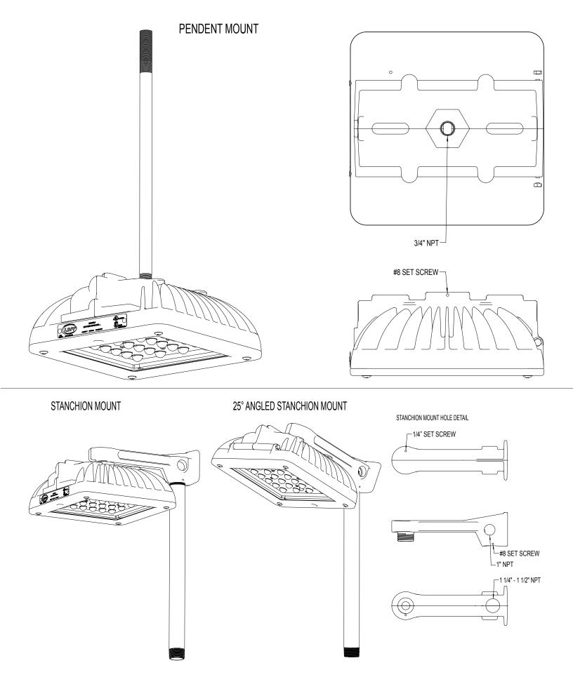
Securely tighten set screws when desired fixture orientation is achieved and the conduit connection is tight.
