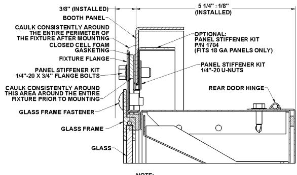
NOTE: LIGHT FIXTURE GLASS FRAME EXTENDS 3/8" INTO BOOTH WHEN MOUNTIED IN BOOTH PANEL
