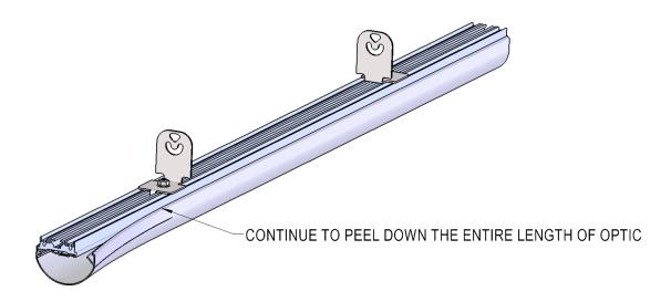
ii. WHEN OPTIC IS REMOVED LED MODULE WILL NO LONGER BE SECURE! 1. BE CAREFUL OF LED MODULE FALLING!
